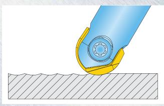
"Sturz" milling, or tilting the axis of the spindle to move the axial center of a ball nose end mill out of the cut, greatly reduces the cutting forces being generated on the nose insert. This shift also relocates the weakest cutting edge geometry out of the way. When allowable in an application "Sturz" milling substantially increases tool life and the quality of finish.
