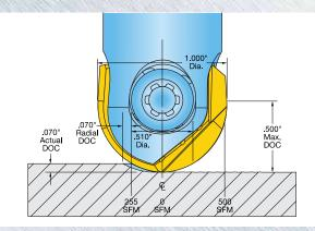
In this example, the SFM is 500 with a 1.000" ball nose diameter. The effective cutting diameter is .510", at which point, the SFM is 255. The RPM must be increased to 3745 in order to achieve 500 SFM at the .510" effective cutting diameter.
